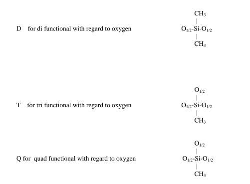
Clearly, there are no real ½ O. This nomenclature is used so that when two or more groups are linked together a single oxygen exists between them. For example MM is often referred to as 0.65 viscosity silicone fluid or hexamethyl disiloxane. Its structure is:
